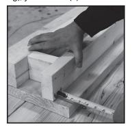
PLACE SUPPORTS: Place support 2"x 4"s atop 2"x 12" (upside down), measure 2-1/4" inches from each side with a 3-3/4" spacer block in between.
